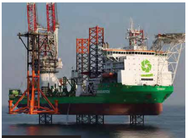
Transport and installation of P11-E minimum facility platform, The Netherlands
