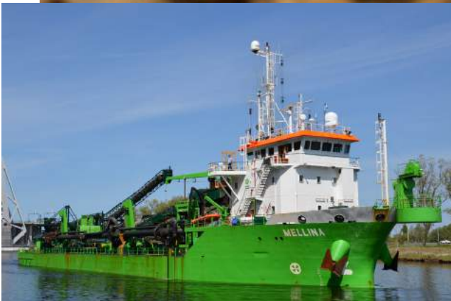
'Mellina' 'Mellina' converted from a hopper into a dry-discharging aggregate dredger
