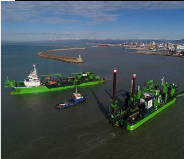
Livorno - Italy TSHD 'Breughel' and CSD 'Amazone' dredging in the port of Livorno
