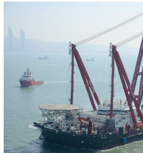
'Gulliver' will have a lifting capacity of 4,000 tonnes
