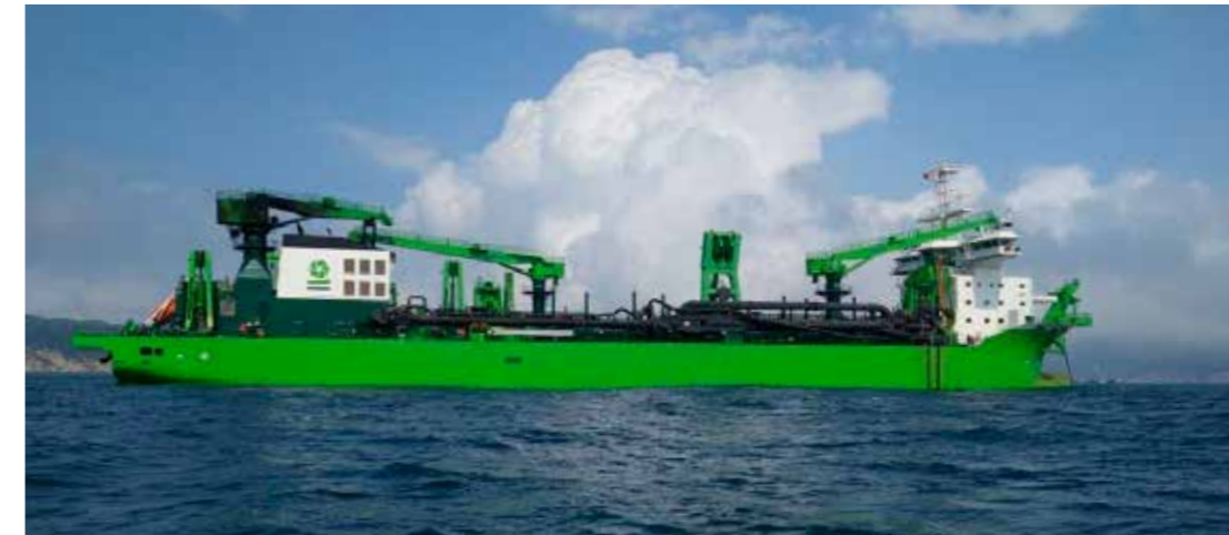
Trailing suction hopper dredger 'Bonny River'
